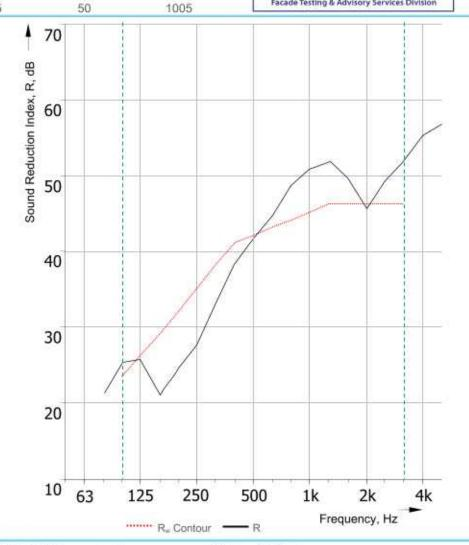
Rating according to BS EN ISO 717-1:2020, over the frequency range 100 Hz - 3150 Hz:
