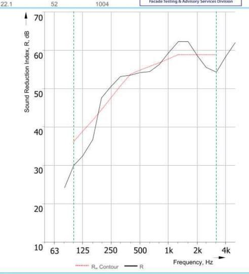
Rating according to BS EN ISO 717-1:2020, over the frequency range 100 Hz - 3150 Hz:
