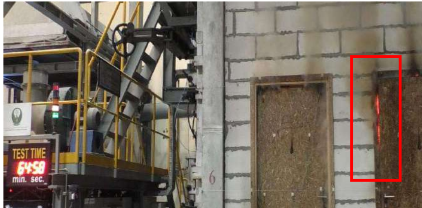
Photo 9. 64 58 minutes of the test. Sustained flaming at the upper left vertical edge of the leaf – Door 2.
