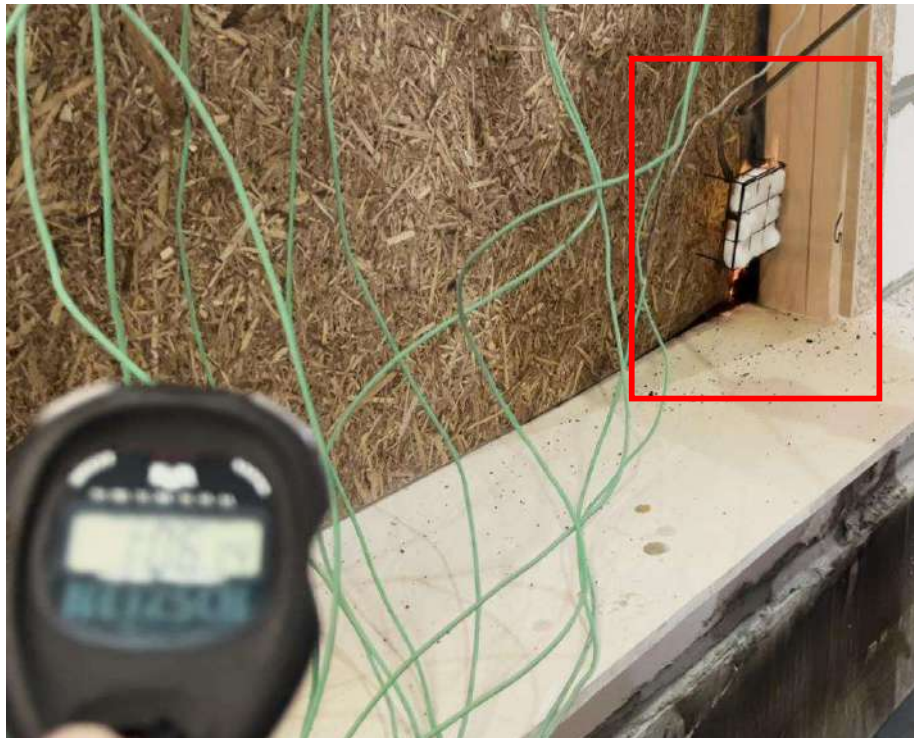
Photo 10. 66 14 minutes of the test. Cotton pad ignition at the bottom right vertical edge of the leaf – Door 1.
