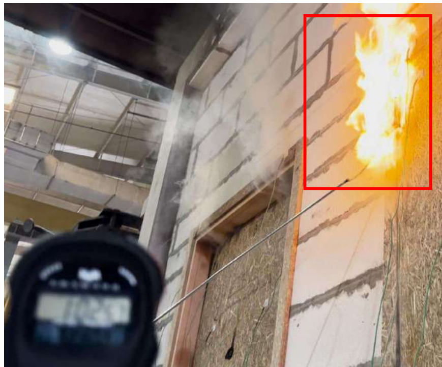
Photo 8. 62 57 minutes of the test. Cotton pad ignition at the upper left vertical edge of the leaf - Door 2.
