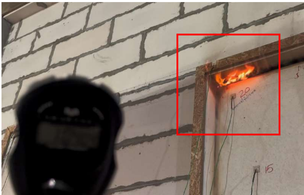
Photo 8. 64 06 minutes of the test. Integrity failure. Sustained flaming at the top left corner of the leaf - Door 18.
