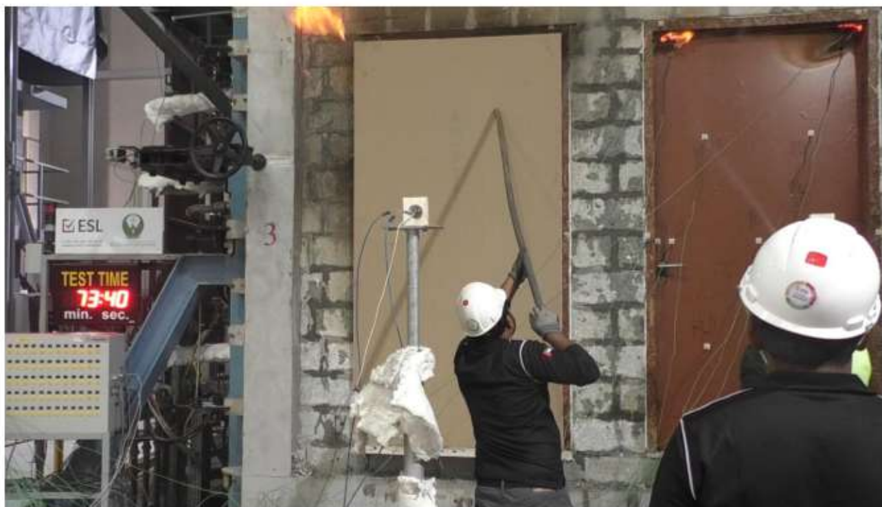
Photo 6. At 73:40 minutes after Door #2 has failed due to sustained flaming from top left corner
