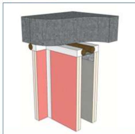
FS702 Intumastic plasterboard to concrete linear gap seal with PE backer rod: EI120
