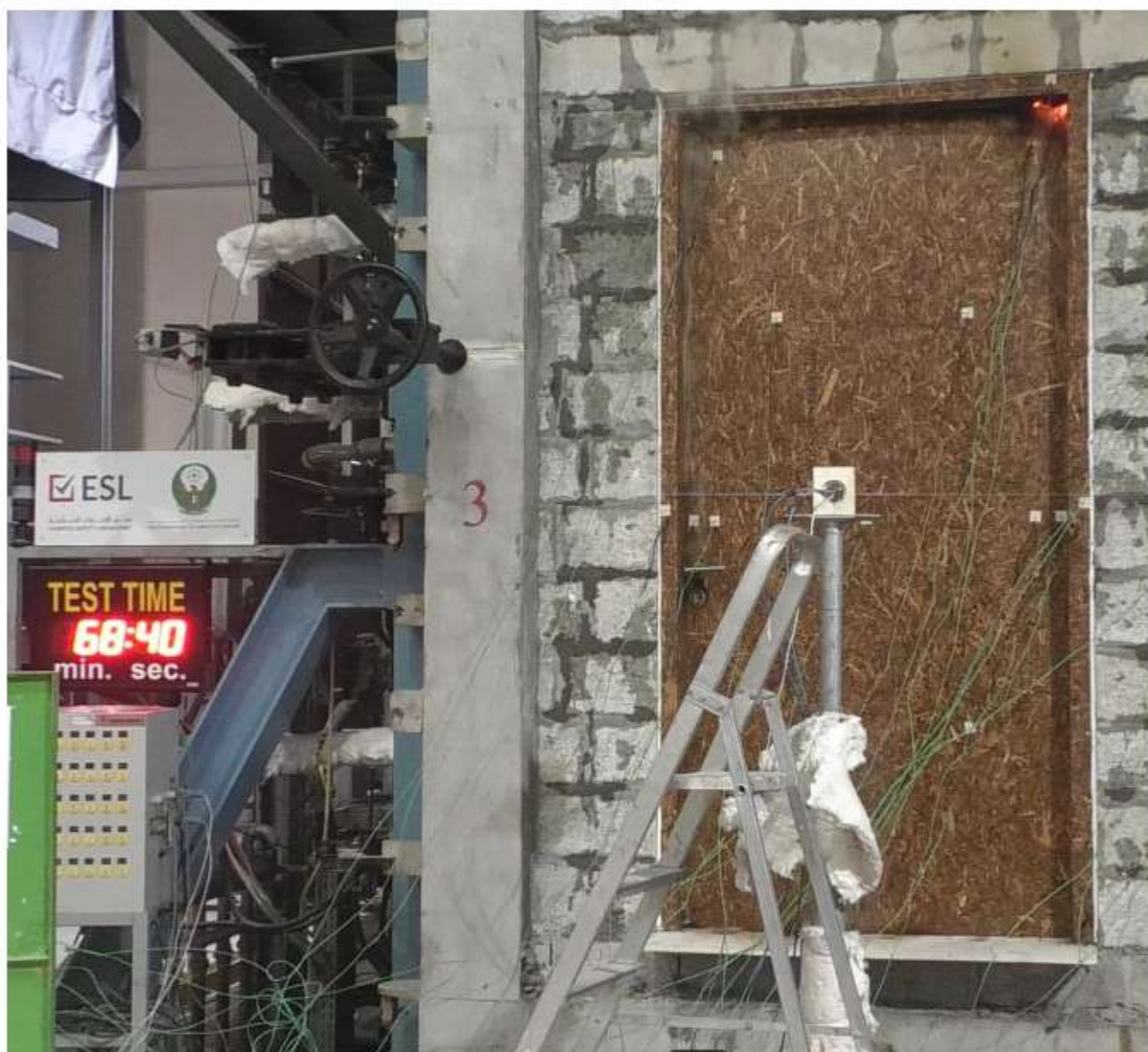
Photo 5. At 68:40 minutes after Door #1 has failed due to sustained flaming.
