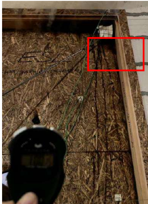
Photo 16. 60 15 minutes of the test. Sustained flaming at the top right vertical edge
