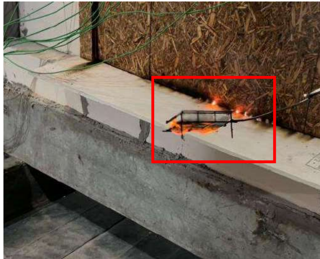
Photo 7. 68 32 minutes of the test. Cotton pad ignition at the door sill
