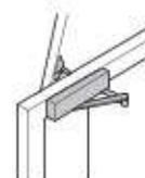
Overhead installation (transom fixing) on push side
