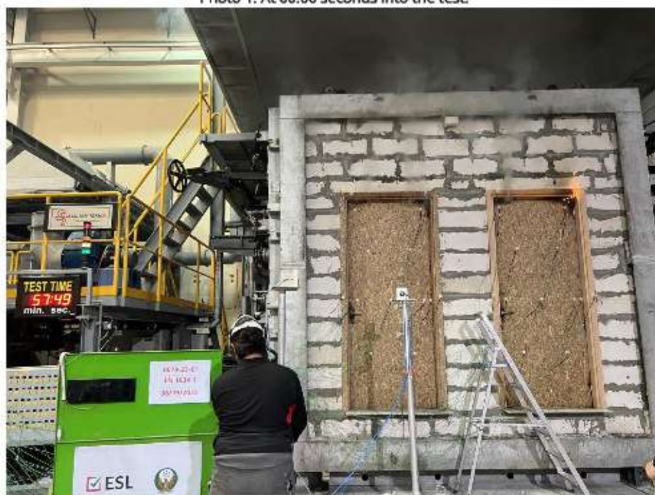
Photo 2. At 57:49 minutes after Door #1 has failed due to ignition of the cotton pad.
