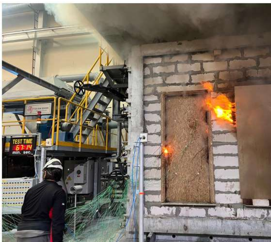
Photo 3. At 67:14 minutes after Door #2 has failed due to sustained flaming.
