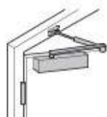
Standard installation (door leaf installation) on pull side
