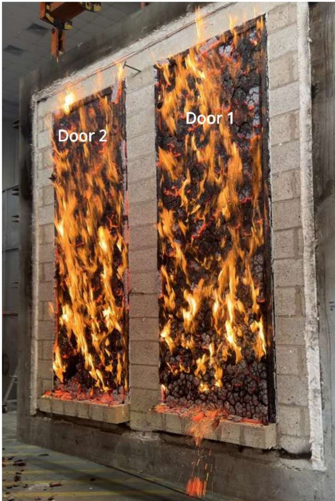
Photo 8. End of the Fire Endurance Test and prior to the Hose Stream Test, while on transit.
