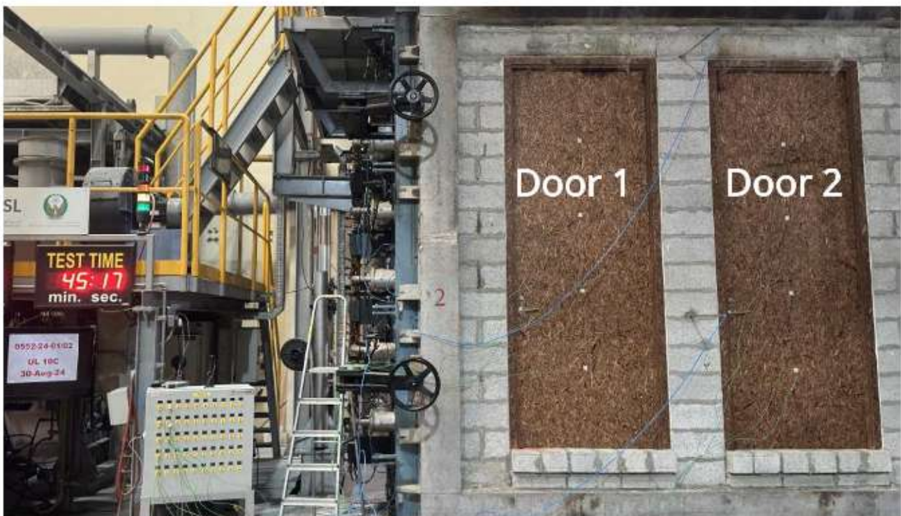
Figure 8. 45minutes of the fire endurance test.
