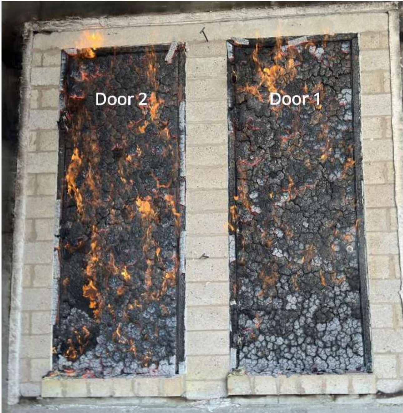
Figure 10. Prior to the hose stream test.
