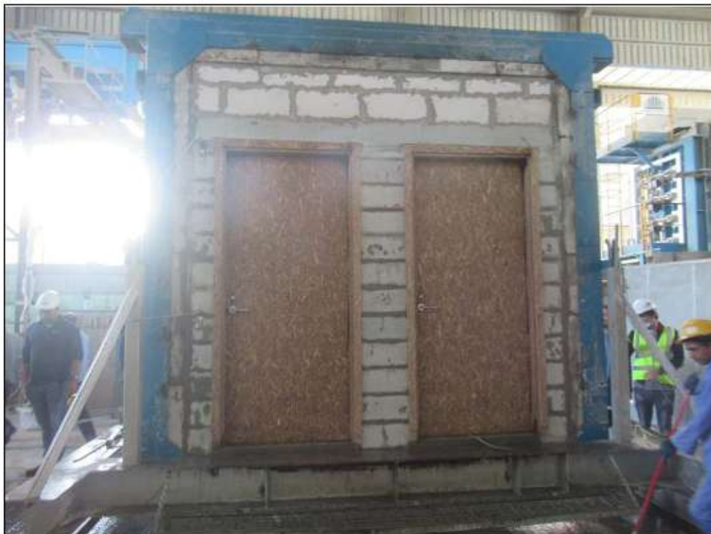
Picture 12: Unexposed face of the specimens after the termination of the hose stream test.
