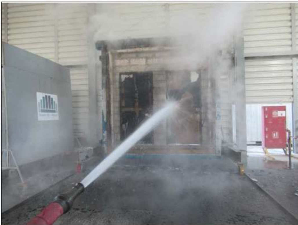
Picture 10: Exposed face of the specimens during the hose stream test.
