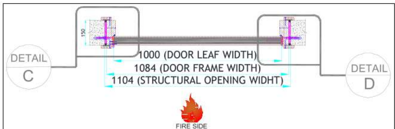
Drawing 4: Horizontal section view of the doorset A. (Drawing provided by the test sponsor)
