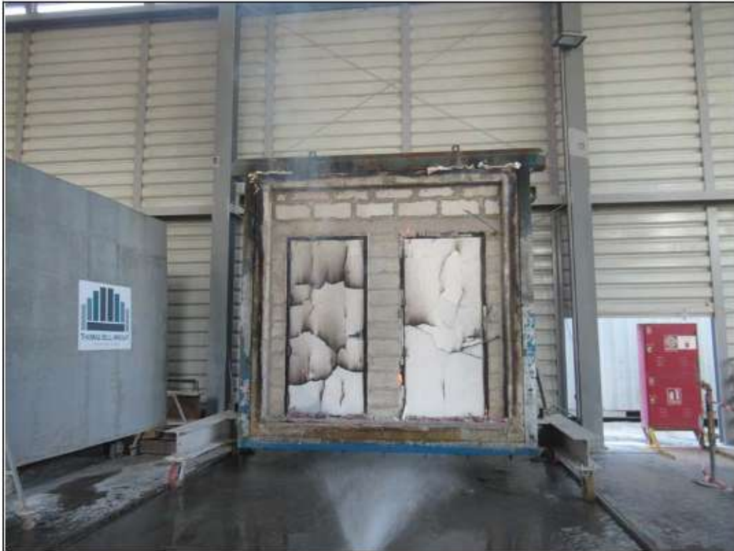
Picture 9: Exposed face of the specimens after the termination of the test.
