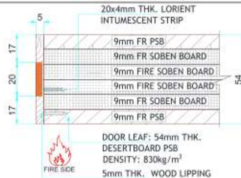
Hinge & Latch Stile Edge and Top & Bottom Horizontal Detail – Doorset A
