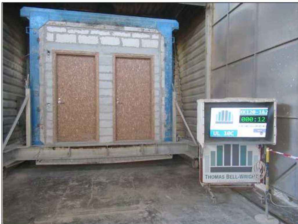
Picture 3: Unexposed face of the specimen at the commencement of the test.
