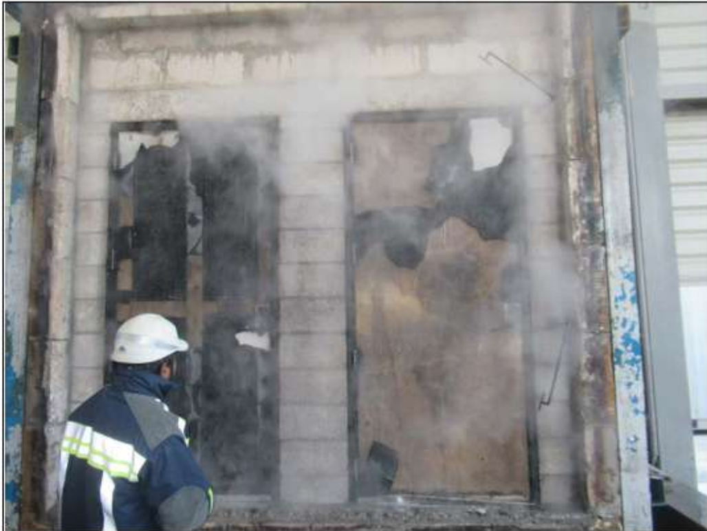
Picture 11: Exposed face of the specimens after the termination of the hose stream test.
