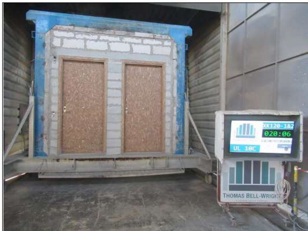
Picture 5: The specimen at 20:00 minutes.
