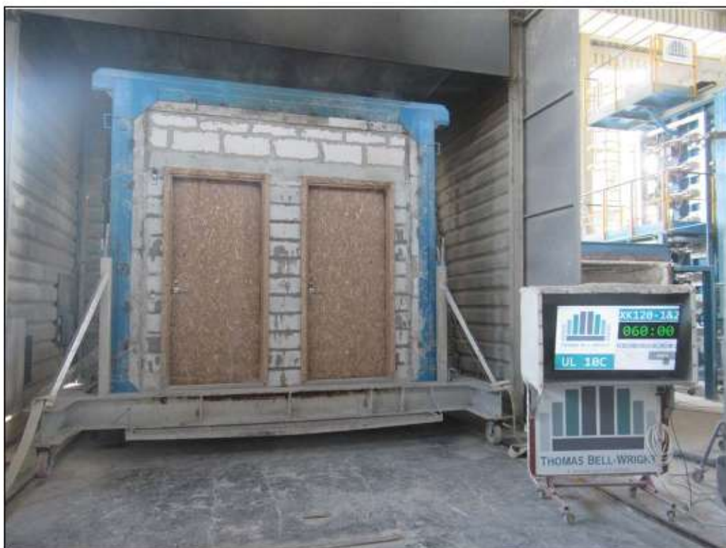
Picture 8: Unexposed face of the specimens after the termination of the test at 60:00 minutes.
