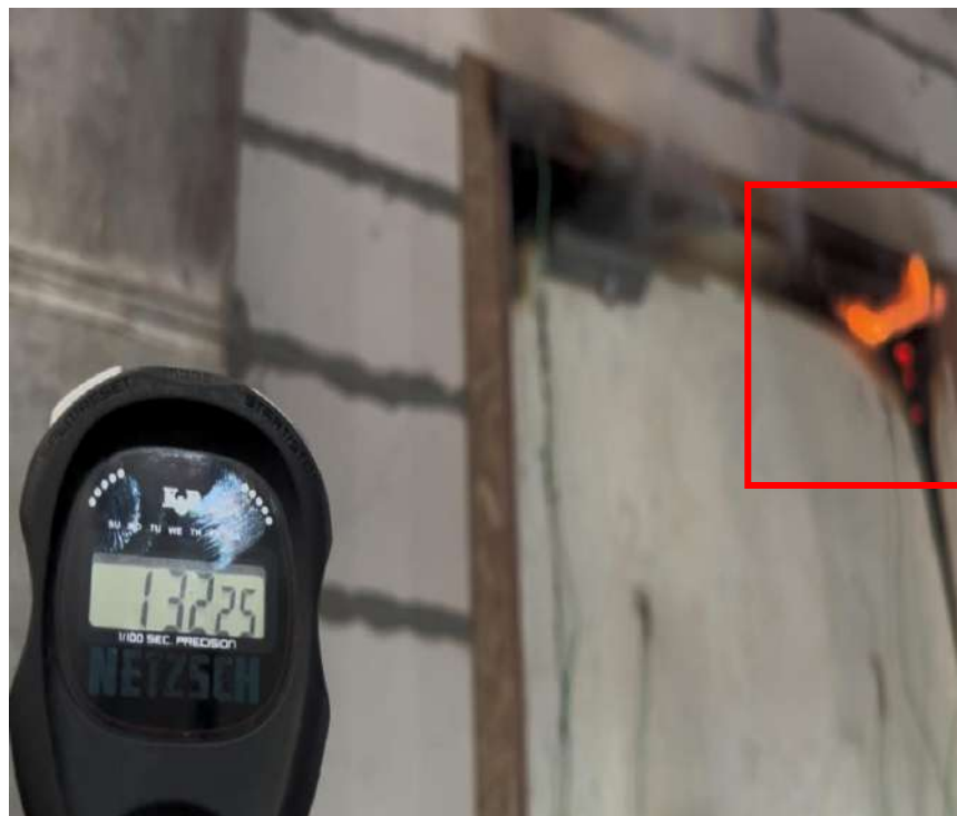
Photo 12. 92 25 minutes of the test. Sustained flaming at the top right corner of the leaf- Door 5.
