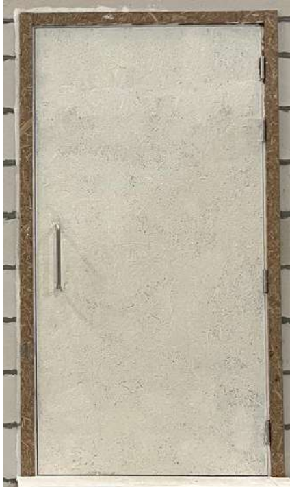
FCC-9000 Flame Core Coat at Door 5 (exposed side)
