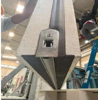
Graphite Liner and Drop-down seal at the Bottom of the Door Leaf
