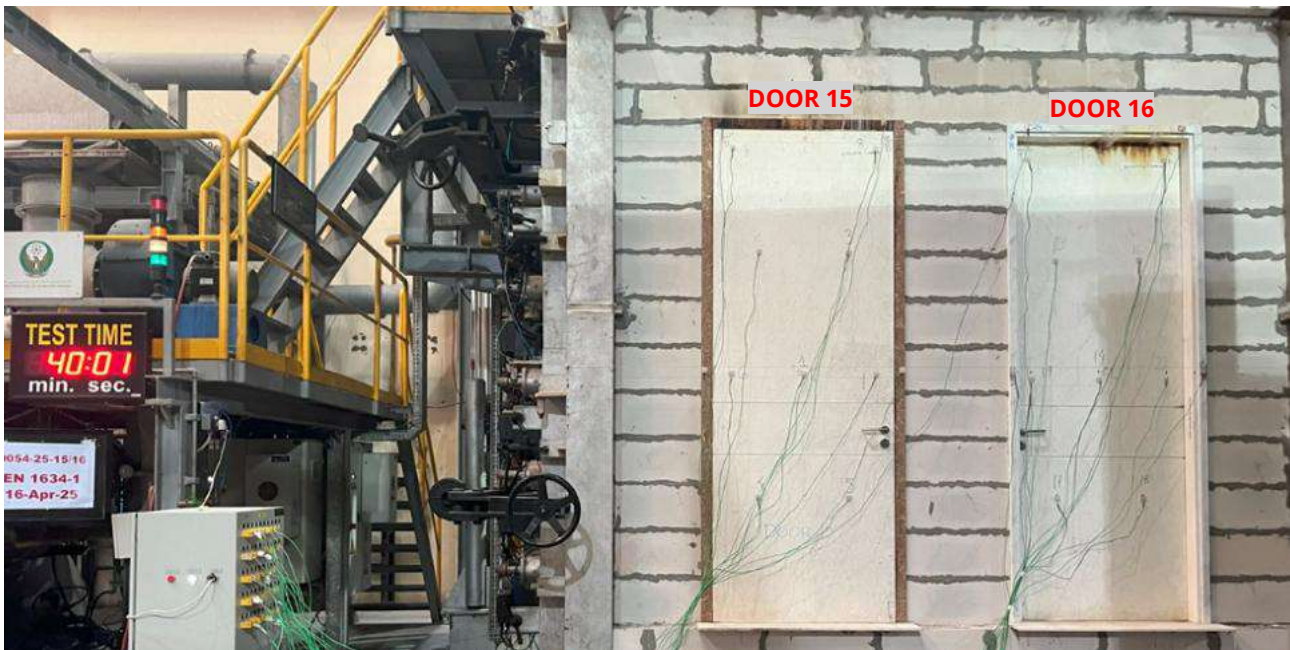
Photo 5. Test specimen at 40-minutes
