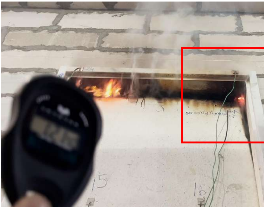
Photo 10. 81 40 minutes of the test. Integrity failure. Sustained flaming at the upper right corner of the leaf – Door 16.
