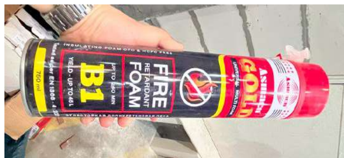
Foam used to fill the gap between supporting construction and frame
