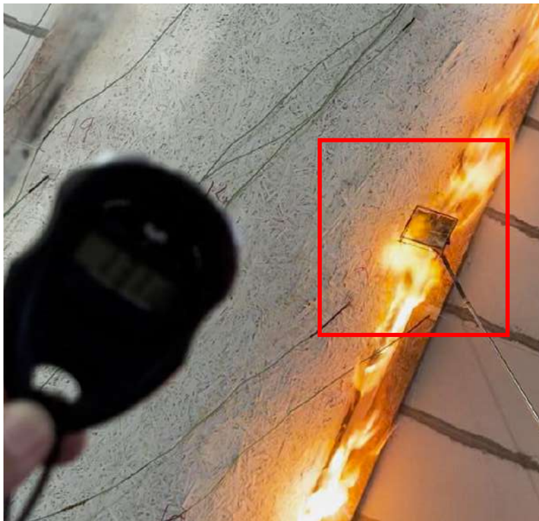
Photo 10. 91 51 minutes of the test. Integrity failure. Ignition of cotton pad at mid-right vertical edge of the leaf – Door 26.
