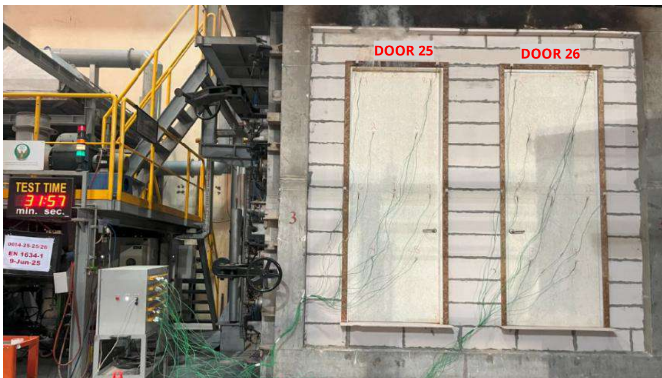
Photo 4. Test specimen at 31-minutes.
