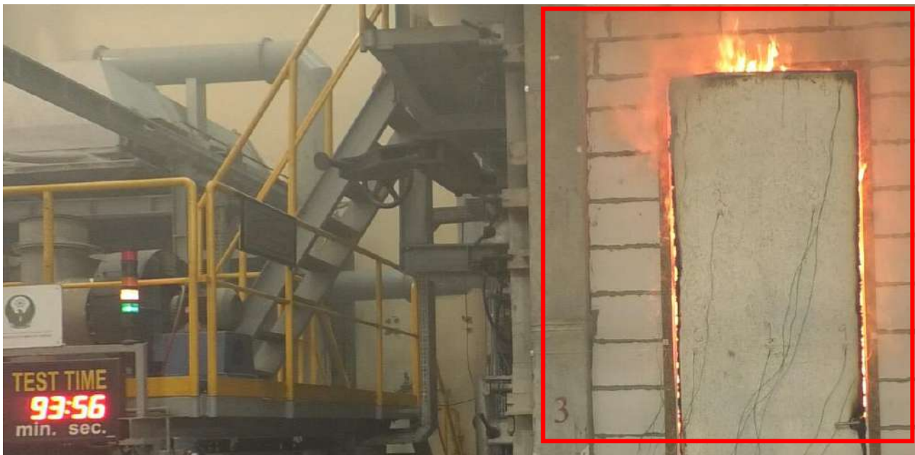
Photo 13. 93 57 minutes of the test. Integrity failure. The upper section of the leaf was detached from the frame and had begun to fall away from the furnace, resulting in a gap that exceeded 25 mm – Door 25.
