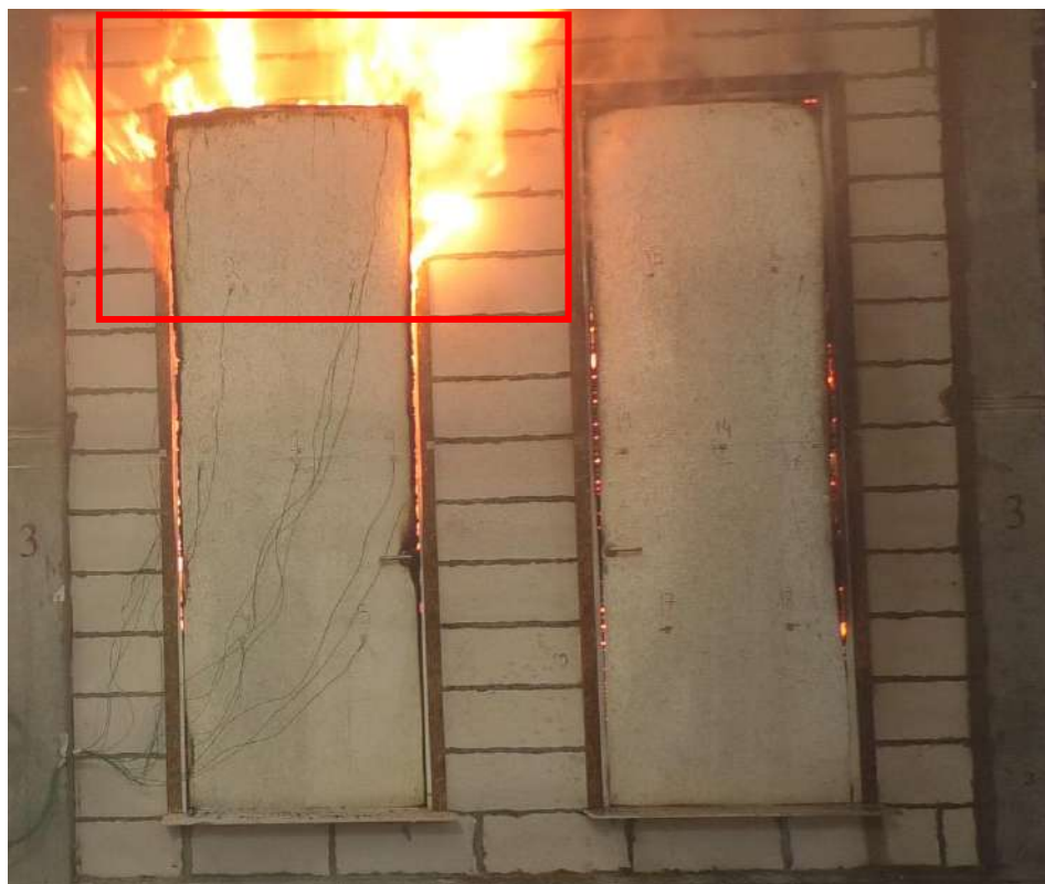
Photo 14. 94 06 minutes of the test. Integrity failure. Sustained flaming on the horizontal top edge of the leaf – Door 25
