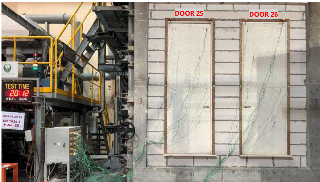
Photo 3. Test specimen at 20-minutes.
