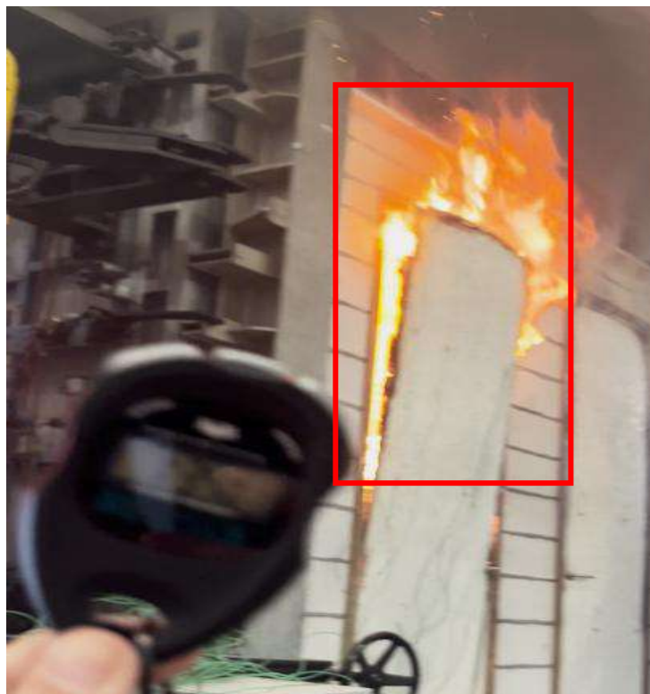
Photo 12. 94 01 minutes of the test. Integrity failure. The upper section of the leaf has been detached from the frame and is falling away from the furnace – Door 25
