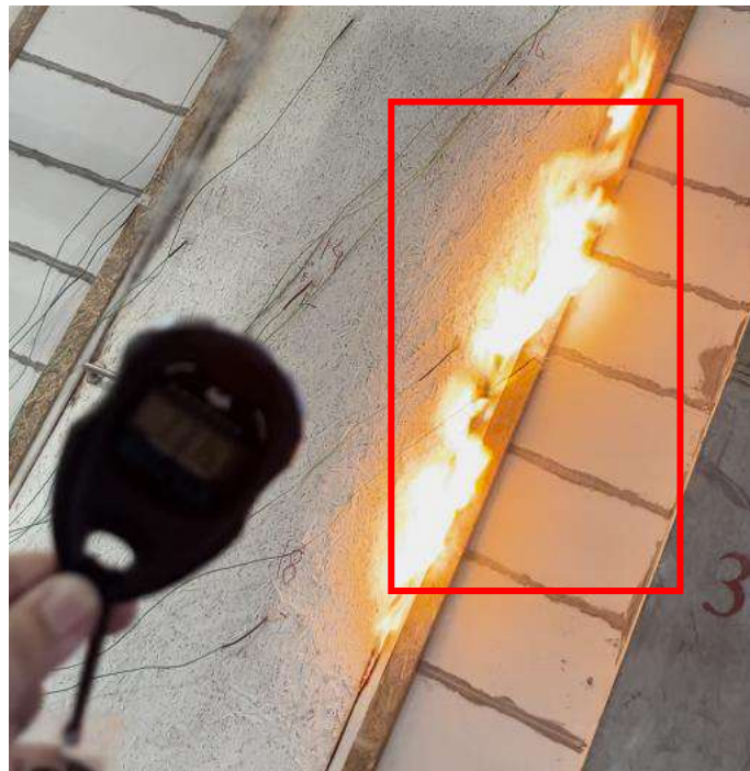
Photo 11. 91 51 minutes of the test. Integrity failure. Sustained flaming at mid-right vertical edge of the leaf – Door 26.
