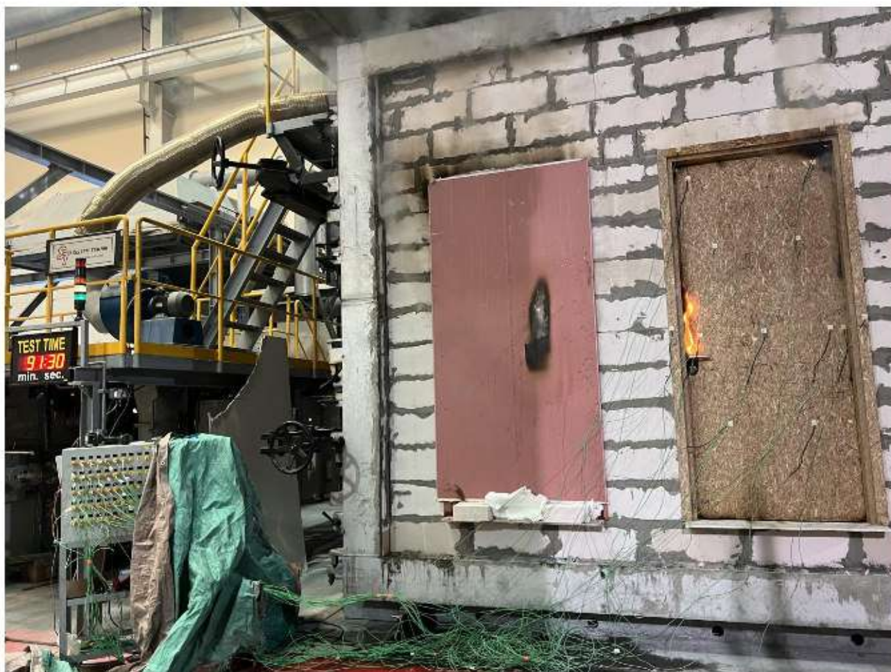
Photo 3. At 91:30 minutes after Door #2 has failed due to sustained flaming.
