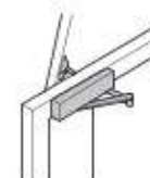
Overhead installation (transom fixing) on push side
