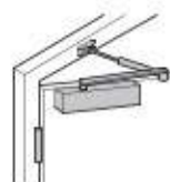
Standard installation (door leaf installation) on pull side
