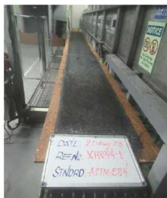
Photo 3: Specimen after the test. (As seen from the fire-end)
